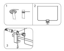
1.Replace the heating wire for bow (Fig.1&Fig.2&): Please wind the heating wire for 4-5 circles in the grooves at both ends of the bow, when winding, please slightly tighten the hot wire tip. After winding, the bow is about 170mm
